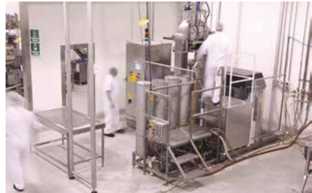
CSIRO Food & Nutritional Science's 35L high pressure processing plant. Image: CSIRO
