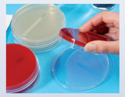
Incubate the plates in an inverted position under conditions appropriate for the test organism.
